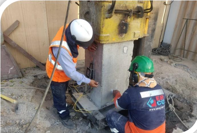
PRUEBA DE CARGA DINAMICA ASTM D4945
